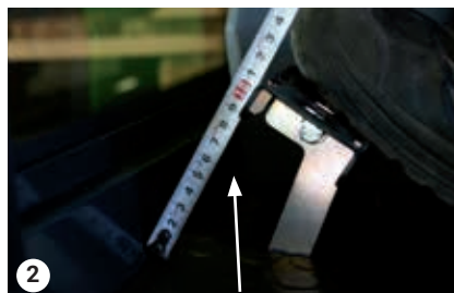
Kontroller pedalvandring 3-5 cm
