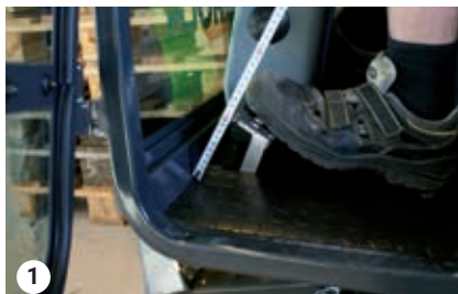
Kontroller pedalvandring 3-5 cm
