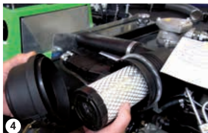
4 Luftfilterelement tages ud
