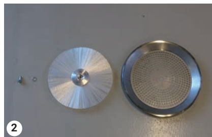
2 Bolt, skive, rotorfilter, rotorrist
