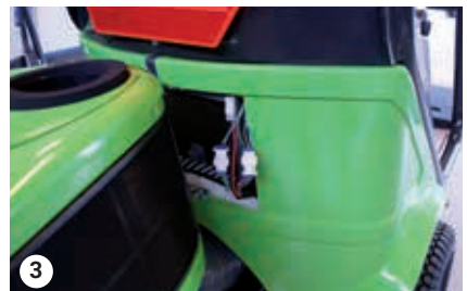
3 3 connectors behind grate
