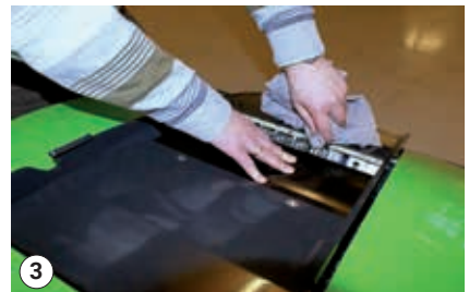
3 Clean the snap couplings – B-frame
