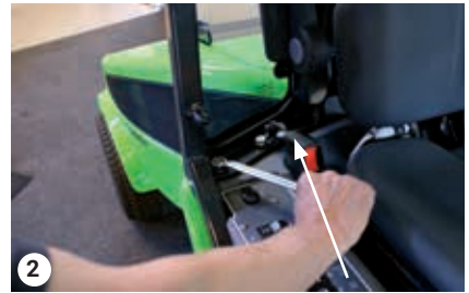
Loosen the 2 bolts on each side
