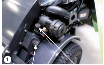
Hydraulic oil – sight glass Filling cap
