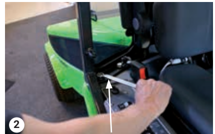
2 Insert the 2 bolts on each side
