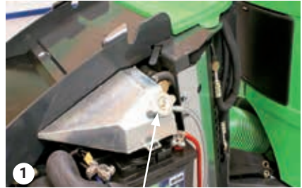
Cooler cover on cooler tank
