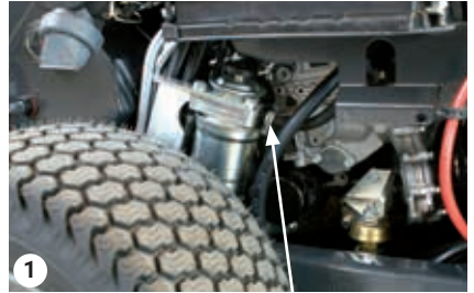
Bleeding screw on the fuel pump
