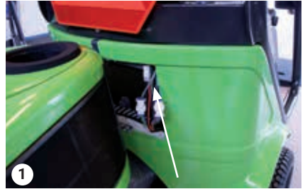
3 connectors behind grate
