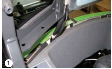
Pull out the cables
