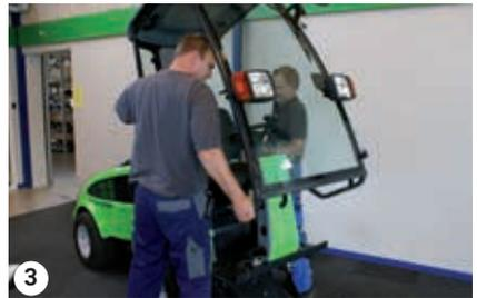
Lift off cab/roll bar
