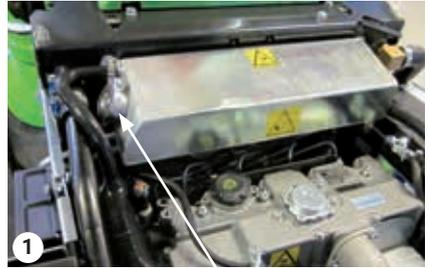
Cooler cover on cooler tank
