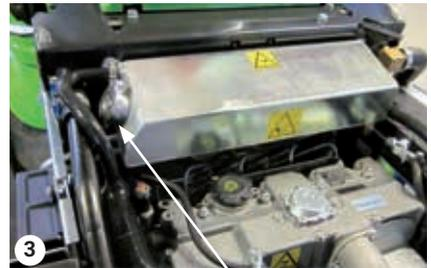
Expansion tank – check coolant
