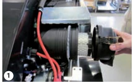
Air filter housing / Filter element
