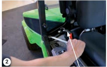
Loosen the 2 bolts on each side
