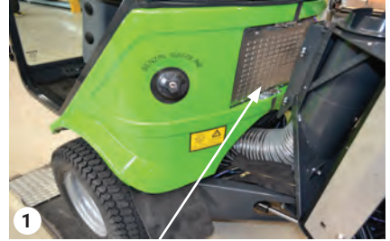
Cabin filter behind grate
