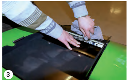
3 Clean the snap couplings – B-frame
