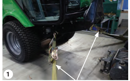
Anchoring at the front
