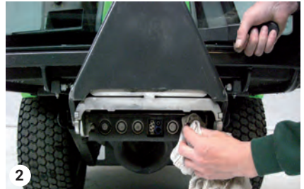
2 Clean the snap couplings – A-frame
