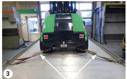
Anchoring at the rear
