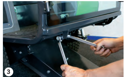
Bolts under base plate
