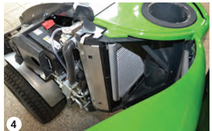
4 Clean coolers using compressed air
