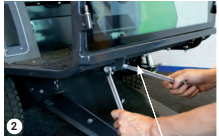
Bolts under base plate
