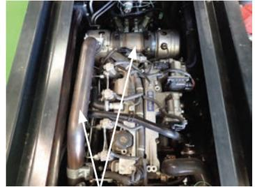
Exhaust pipe line and D.O.C
