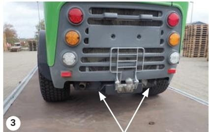
Anchoring at the rear, two anchor brackets
