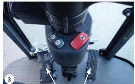
Inching/brake pedal Drive pedal
