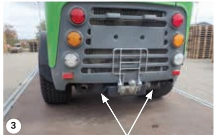
Anchoring at the rear, two anchor brackets
