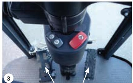
Inching/brake pedal Drive pedal
