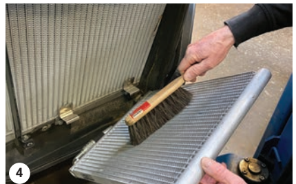
Air conditioning condenser
