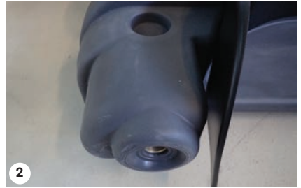
Hydraulic oil drain plug
