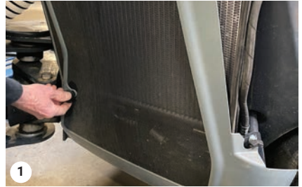
Access to radiator and air conditioning condenser
