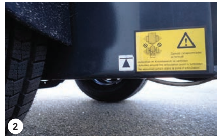
Articulation joint warning
