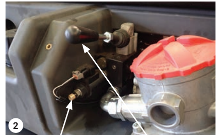
Hydraulic pump valve
