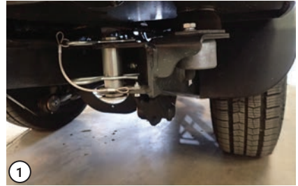
Anchoring at the front
