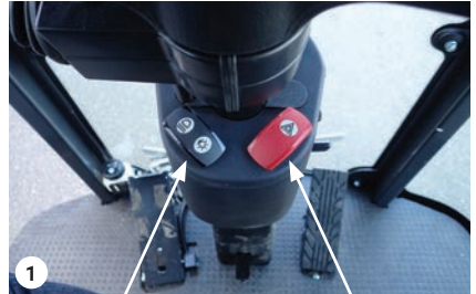
Light switch Hazard switch
