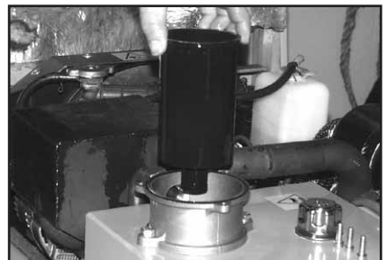
Tank filter housing
