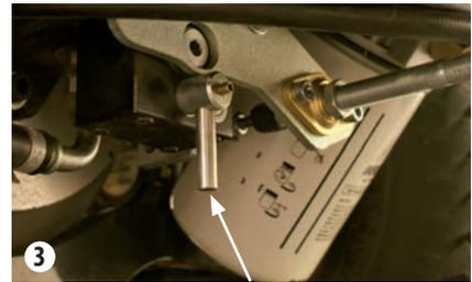
Towing lever in "closed" position
