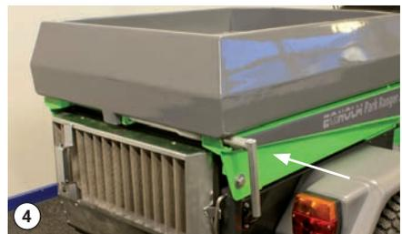
Locking lever in "locked" position
