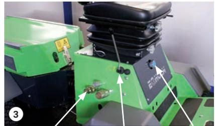
Hydraulic connectors D1, D2, D3 Lever D
