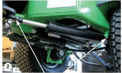
Lubricating nipples, steering cylinders
