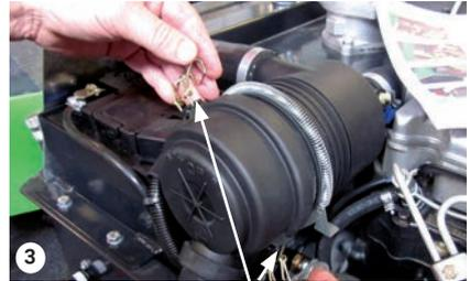
3 Loosen the filter housing
