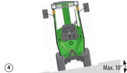
4 Do not drive on slopes with an incline of more than 10°
