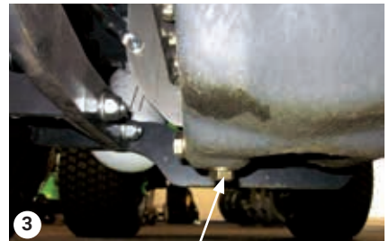
Remove the bottom screw
