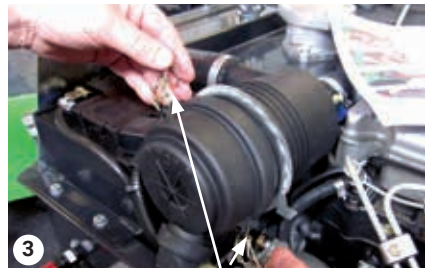
3 Loosen the filter housing
