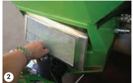
Fitting the oil cooler cover
