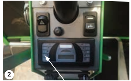
Control light for diesel
