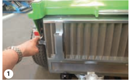
1 Removing the radiator cover
