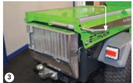
Locking handle in "released" position
