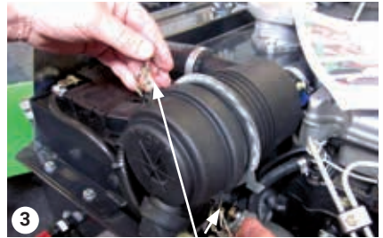
3 Loosen the filter housing
