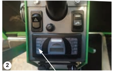
Control light for diesel
