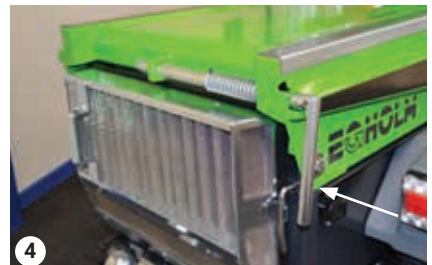
Locking handle in "released" position
