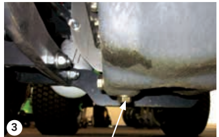
3 Remove the bottom screw
