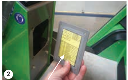
Fuse overview - Back of the fusecover
