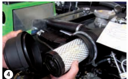
4 Remove the air filter element
