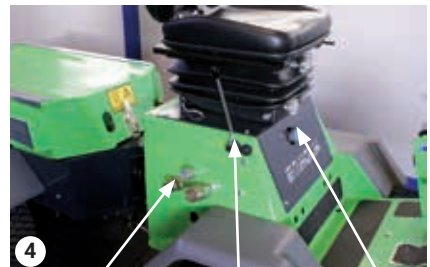
Hydraulic connectors D1, D2, D3 Lever D Speed regulation
