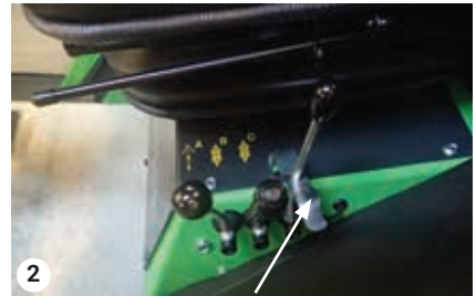
Locking handle for lever C
