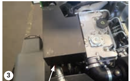
Main fuse - 50 Amp
