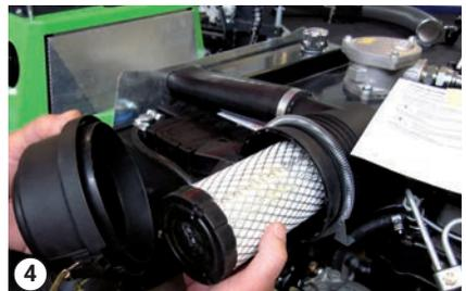
Remove the air filter element
