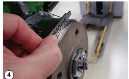
The wheel flange must be outside the bonnet key. If the flange is covered or almost covered the drum must be replaced.
