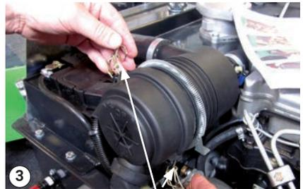
Loosen the filter housing
