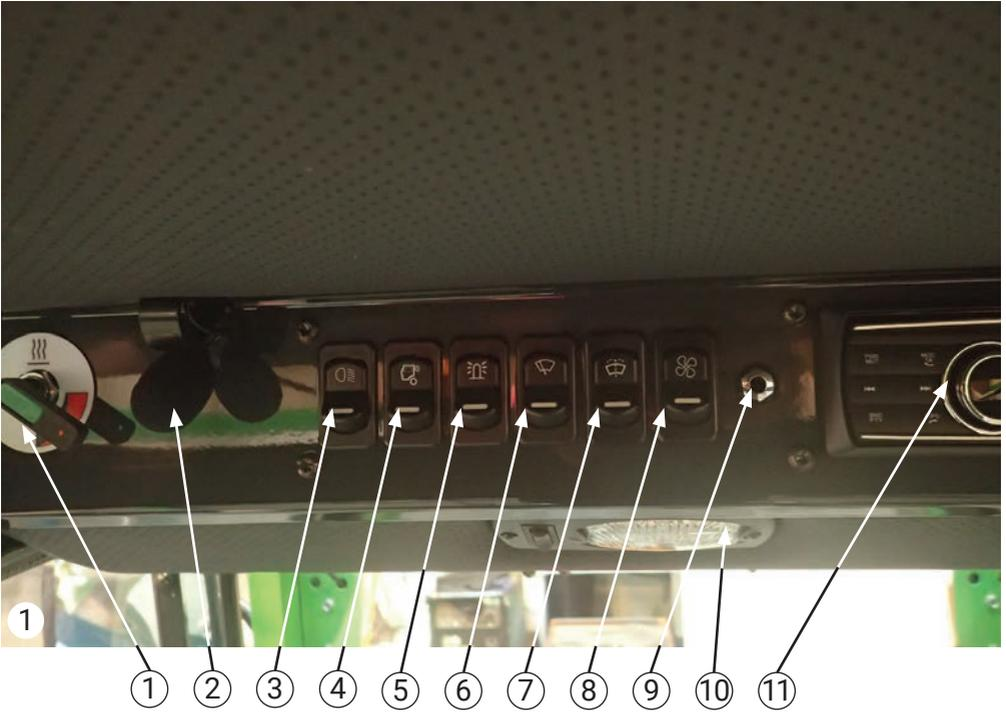
1. Heat regulation in the cab (for heat, turn on red).
