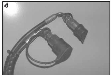
Fit the protective caps onto the snap connectors
