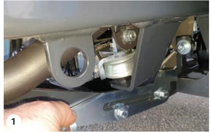
1 Unhook the environmental rake from the rear lifter.
