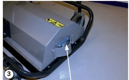
Lubricate the bearing on the right-hand side
