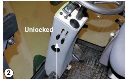
Transport lock in unlocked position
