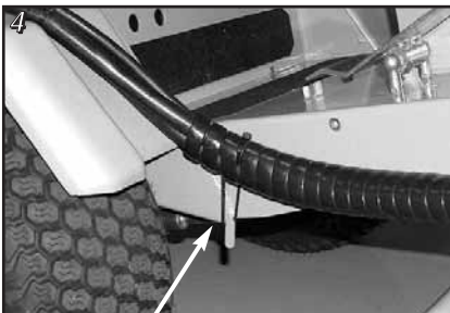
The hoses are fastened with a rubber strap
