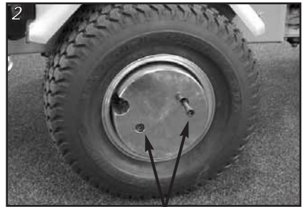
Fit and tighten the counterweights
