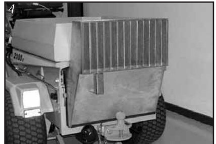
Big radiator cover for the water cooler
