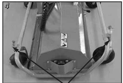
Lubricate the castor wheel forks
