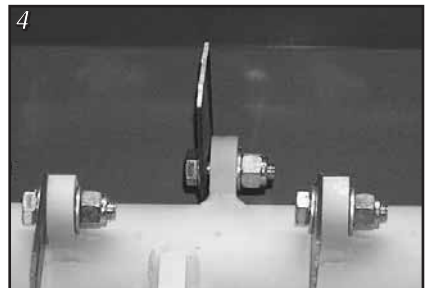
The vertical blades are fitted individually
