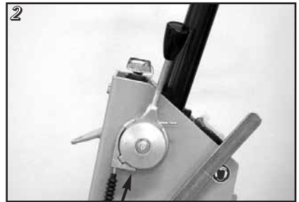
Turn the throttle until it is half open
