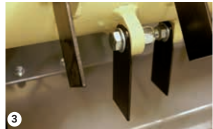
Vertical blades fitted individually
