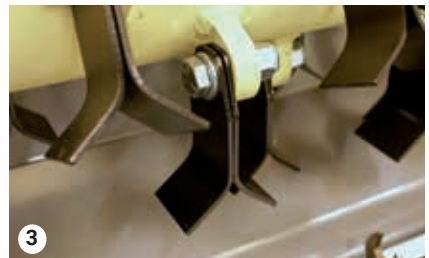
The flails are fitted together
