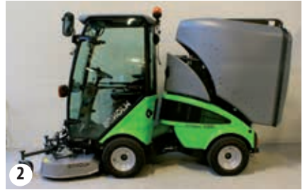
Lowering the hopper
