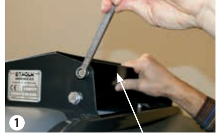
Adjustable vent at the top of the container
