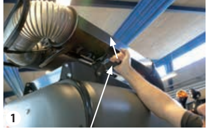
Flip the transport lock up
