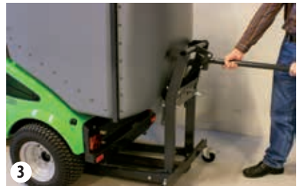
Attaching the hopper
