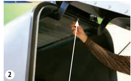
Release top grate at the back
