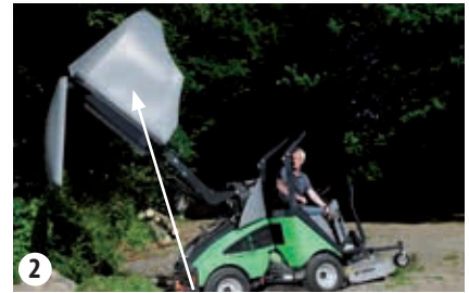
Hopper is tipped as far as it can
