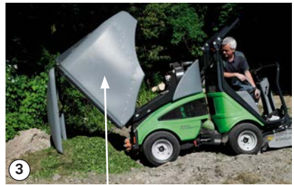
The hopper is tipped back as far as possible
