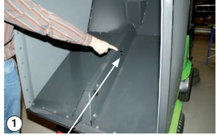
Plastic stopper on the inspection hole
