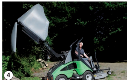
The hopper is raised to max. height and tipped as far back as possible.
