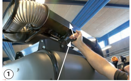
Flip the transport lock up
