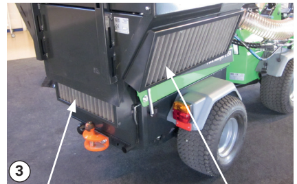
Side air intake filter
