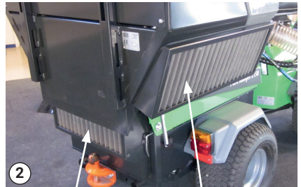
Side air intake filter
