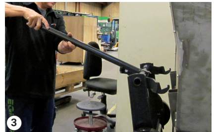
Lowering the hopper
