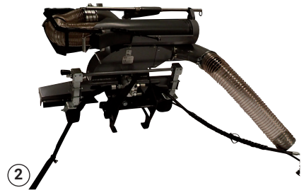
Spread the suction hose and hydraulic hoses out to the sides before attaching
