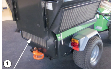
Rear air intake filter
