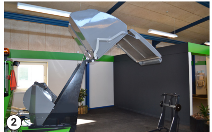
2 Hopper tipped to maximum
