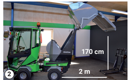
Tipping the hopper
