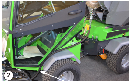
Secure hydraulic hoses - left side
