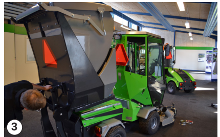
Push first and then lower the hopper over the bonnet
