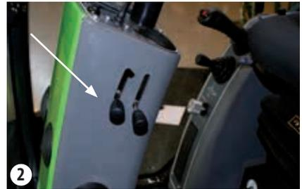
Transport lock in unlocked position
