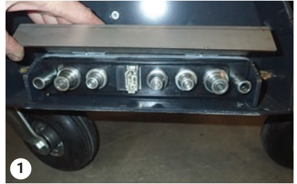
Cleaning the couplings
