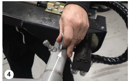
Mount the cutter knife in the square hole, M10 bolt
