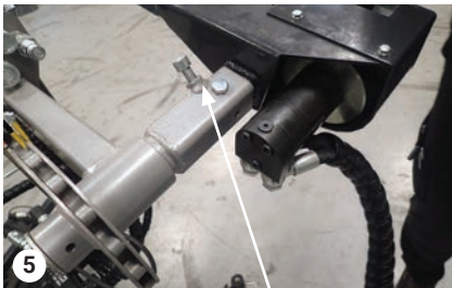
Tighten the allen bolt. Check the cutter can not move at all from the cutter arm square pipe.
