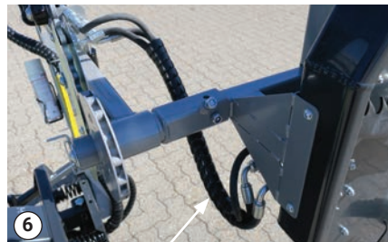
The hydraulic hoses must be guided below the trimmer arm square pipe.
