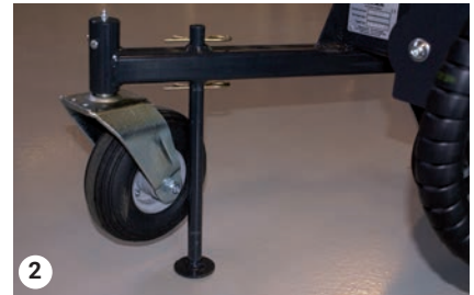
Support strut lowered
