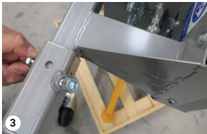
Mount the trimmer knife in the square hole, M10 bolt.
