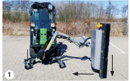
Change cutting bar to right side
