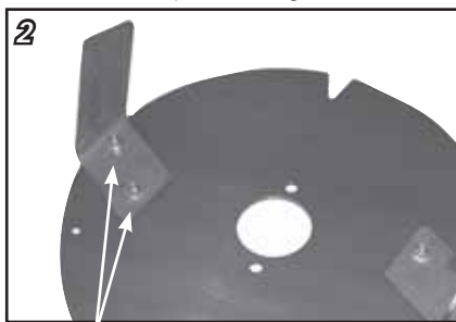
Nuts which hold the blades
