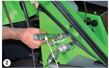
Oil overflow hose at connector D-3
