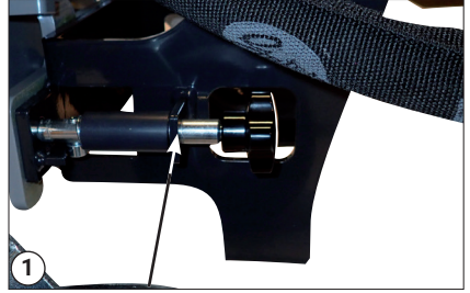
Locking pin open – leaf suction unit in floating position
