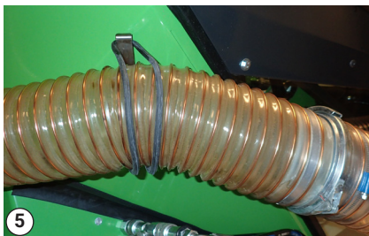
Affix the suction hose using the rubber strap for machines with cab
