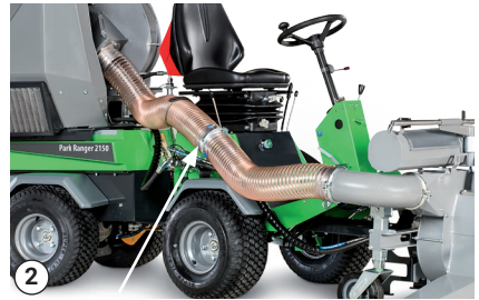
Connect the suction hose using the hose clip
