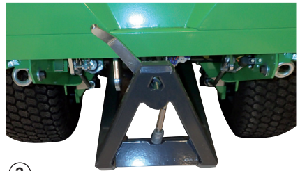
Locking handle on the A-frame, open
