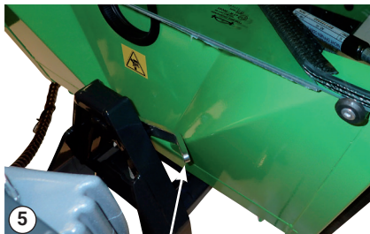
Attachment locking handle in locked position
