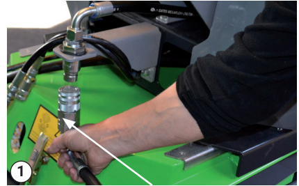
Return hose from the leaf suction unit – with female connector
