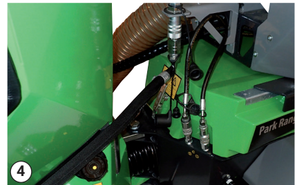
Secure hydraulic hoses - left side
