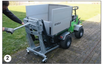
Lower the rear tipper onto the engine cover
