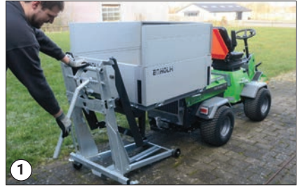
Push the rear tipper to position it above the engine cover
