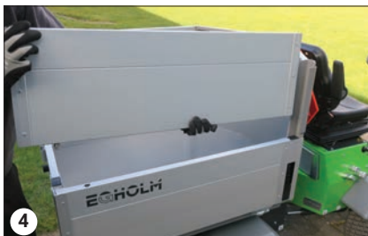
The upper section can be removed separately
