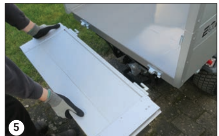
Tailgate and sides can be fully removed
