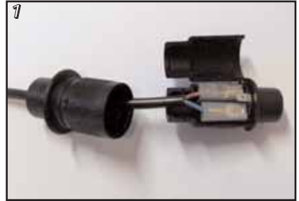
Fit the power connector
