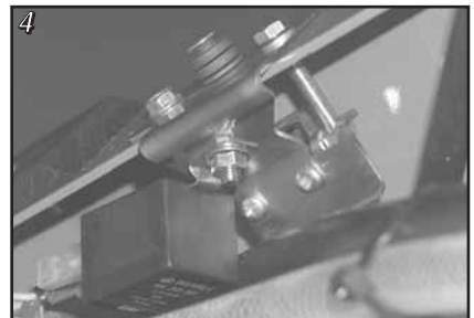
Load cell fitted
