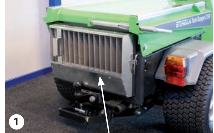
Water cooler cover
