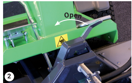
Locking handle on the A-frame – open
