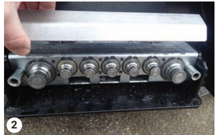
Clean the hydraulic couplings
