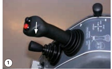
1 Adjustment handle – Raising the cutting height
