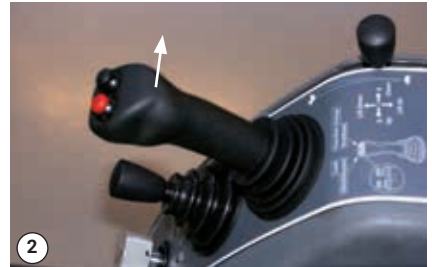
2 Adjustment handle – Lowering the cutting height
