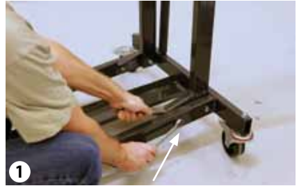
2 bolts on the tank frame
