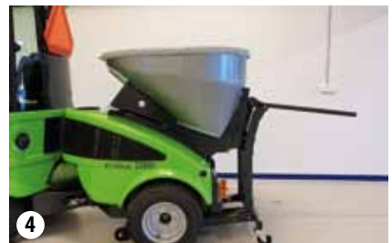
Mounting the Salt and Sand Spreader
