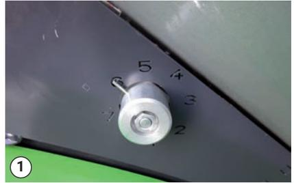
Adjusting the spread width
