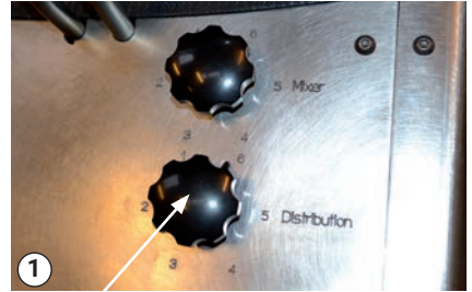
Adjusting the spread width - "Distribution"
