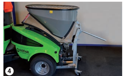
Mounting the salt and sand spreader
