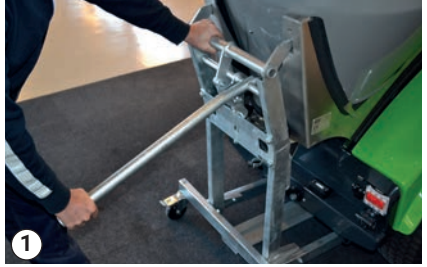
Salt and sand spreader being lowered onto the machine
