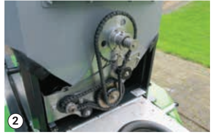
Check and lubricate the chains
