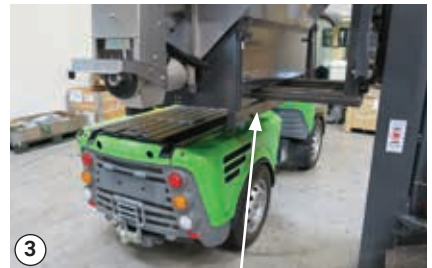
Lifting the Spreader away from the Basic machine
