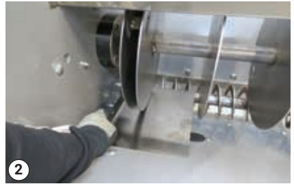
Loosen and remove 3 screws, and install the salt stop by sliding it in from the side
