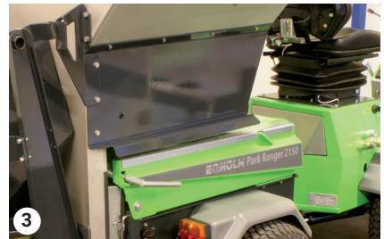
Lowering the salt and sand spreader
