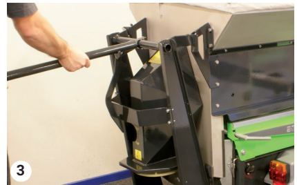
Lower the salt and sand spreader
