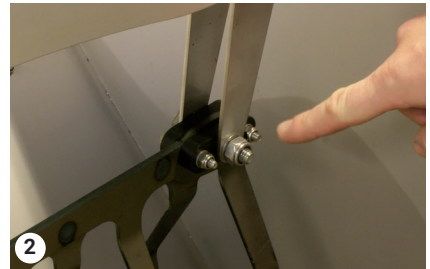
Bolts for the stirrer system
