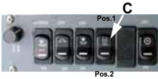
Adjust the ejection door and set the throwing distance by activating the switch (C).
