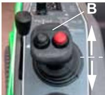
The joystick (B) can be used to lift and lower the snow blower.
