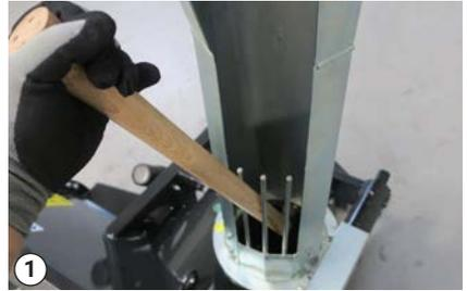
Use the woden bar to unlog the chute
