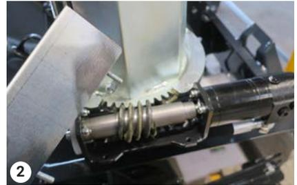
Remove the cover, and grease the worm gear
