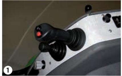
The Dozer Blade is raised using the joystick
