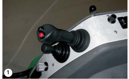
The snow plough is raised using the joystick
