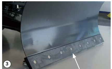
Nuts holding the scraper edge
