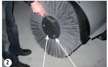
2 Disassembling the flange Bolt
