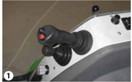
The Snow V-Blade is raised using the joystick
