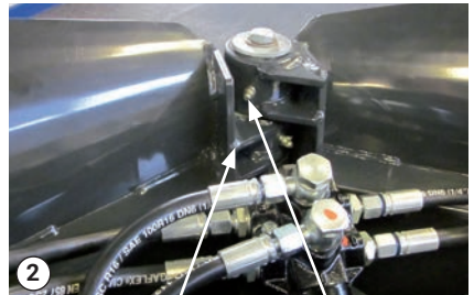
Location of lubrication nipples
