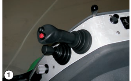
The snow V-plough is raised using the joystick
