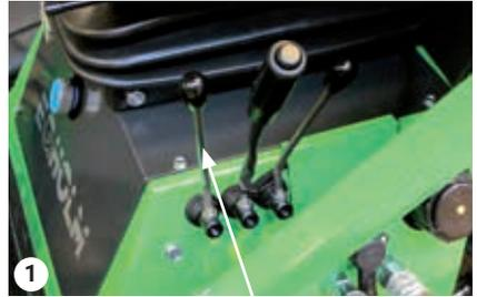
The snow V-plough is raised using lever A
