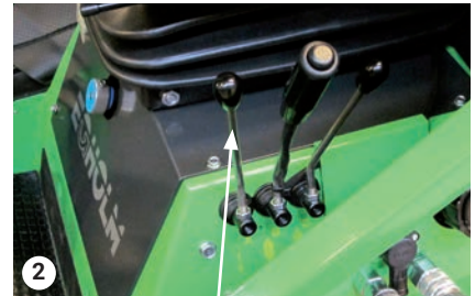
Use lever A to lower the snow V-plough
