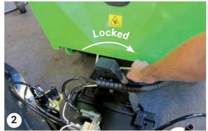
Lock the locking handle on the A-frame
