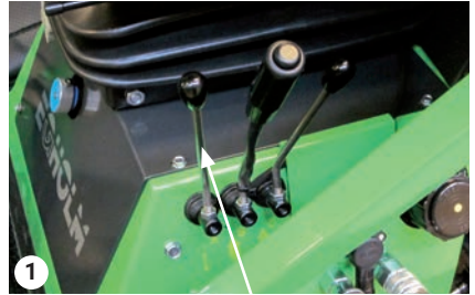
The snow V-plough is raised using lever A
