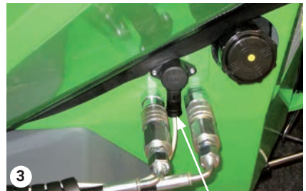
Fit the hydraulic hoses and power plug
