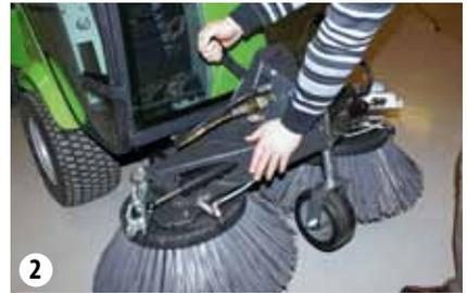
Tilt the attachment into the machine
