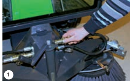
1 Detach the hydraulic hose
