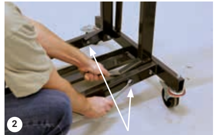
Two bolts on the hopper frame
