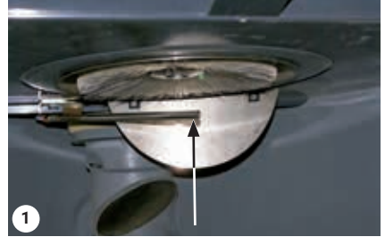
Checking the rotary filter and turbine
