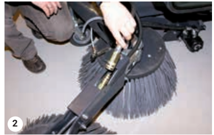
Hydraulic hoses + water hoses on the side-brush are fitted
