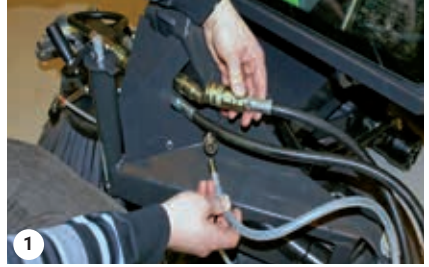
Hydraulic hoses + water hoses on the A-frame are fitted
